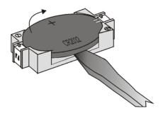
Inset 2: Inserting the New Battery
